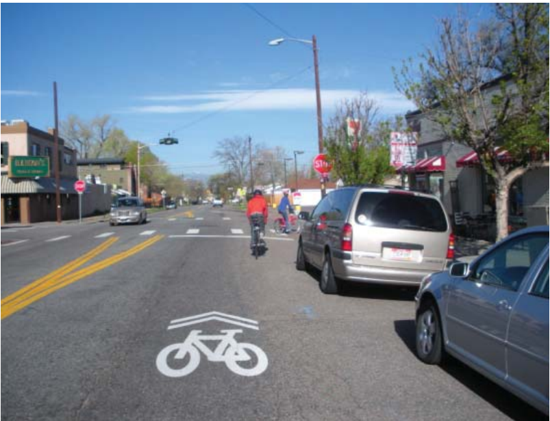
Example of a Class III Bicycle Facility
