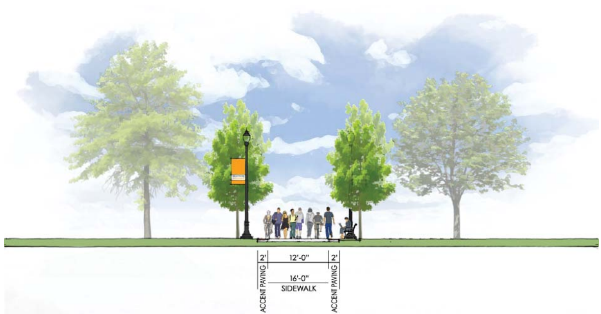
Figure 3.15 - Typical Pedestrian Avenue Section
