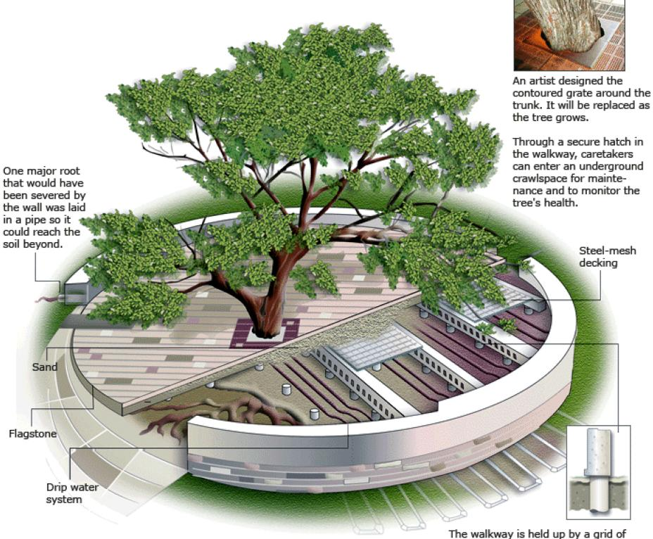
The aeration and watering system is about 3 feet deep at the original grade and extends 15 feet from the wall.
