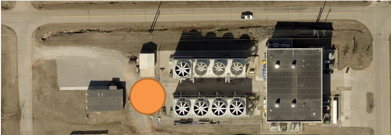
Figure 19, West Chilled Water Plant and Recommended Location of Thermal Storage Tank
