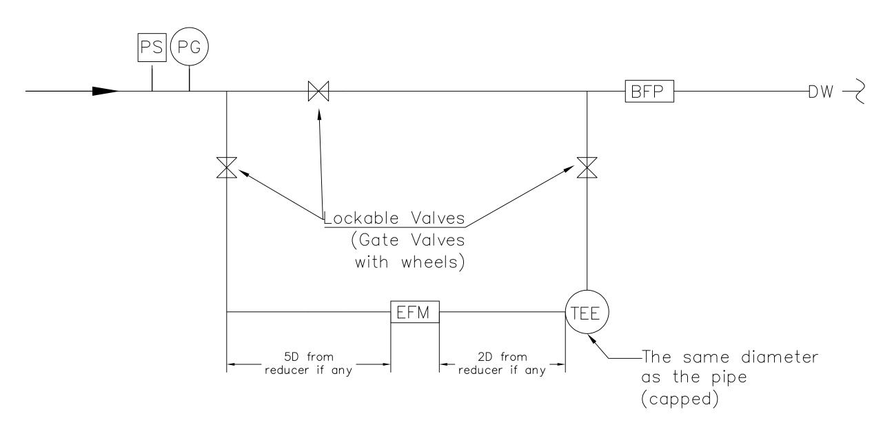
PS: pressure transducer with isolation valve
