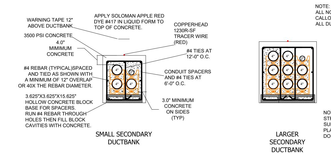
THE DUCTBANK PROFILES SHOWN HERE ARE TYPICAL OF ALL DUCTBANK REQUIREMENTS WITH ADDITIONAL STEEL, CONCRETE BLOCK AND CONCRETE FOR THE LARGER DUCTBANK.
