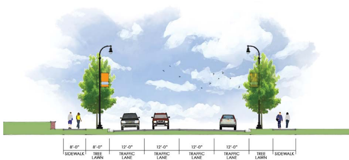
Figure 3.5 - Recommended Duck Street Section
