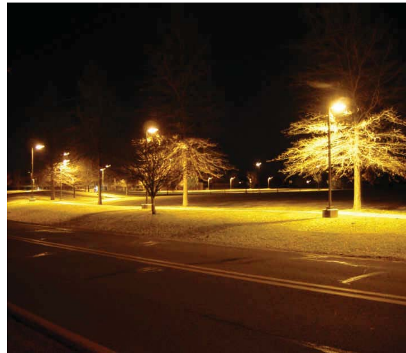
Good example of full cutoff light fixtures directing light efficiently down onto the walkway, which is brightly lit.
